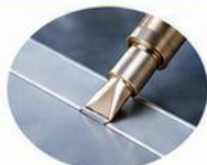
Plastic sheet welding
